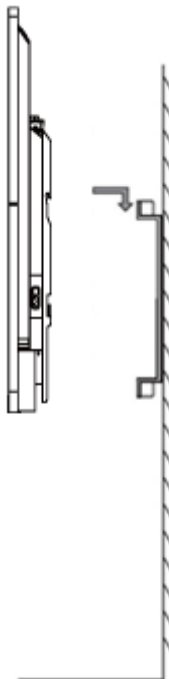
Figure 3-9 Wall Mount Side View
